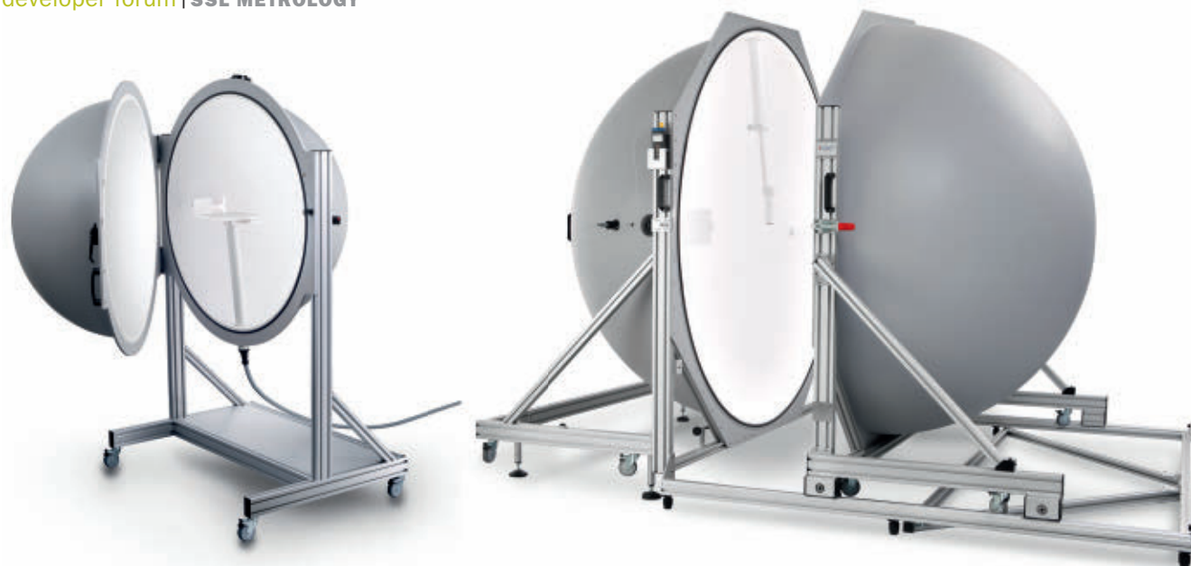
FIG. 2. A 1m-diameter sphere (left) is ideal for measuring most LEDs and modules in the 4\pi and 2\pi recommended geometries. A 2m sphere (right) is ideal for large luminaires and SSL products.
