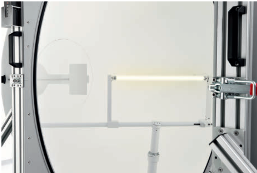
FIG. 4. Example of avoiding near-field absorption effects. The holder of the linear tube is placed as far away as possible from the light source and coated with a high-reflectance material.
