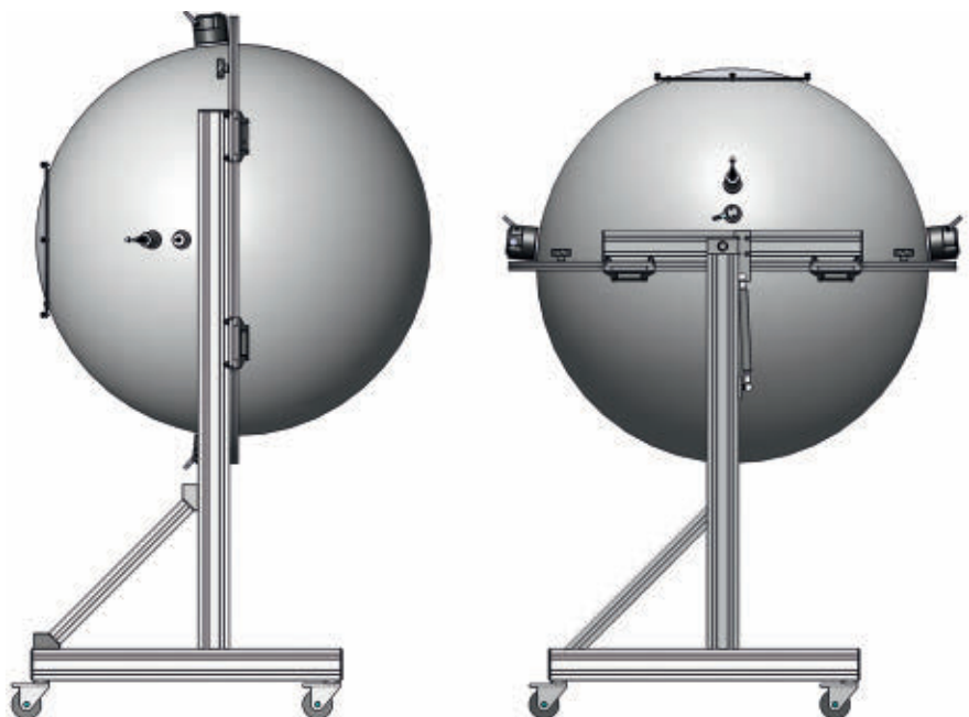
FIG. 5. A rotatable 1m sphere. Position-sensitive light sources can be measured in their designed operating position.
