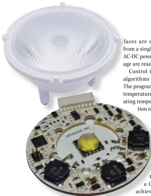
FIG. 4. A compact emitter, secondary optic, and driver control board make it easy to implement halogen-style dimming with all the benefits of LEDs.
